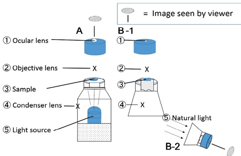
Figure 1. Structure of the MyMicroscope (A) and the PET bottle microscope (B-1) (B-2).
