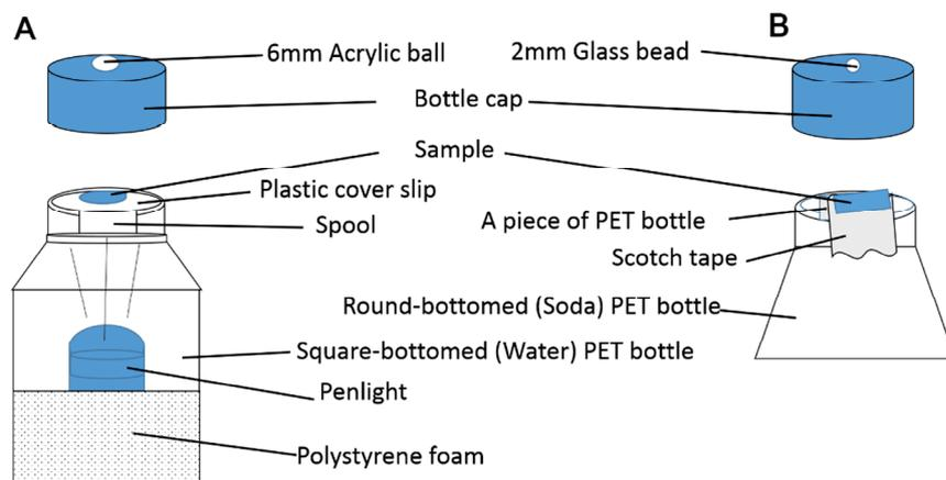
Figure 2. Design of the MyMicroscope (A) and the PET bottle microscope (B).
