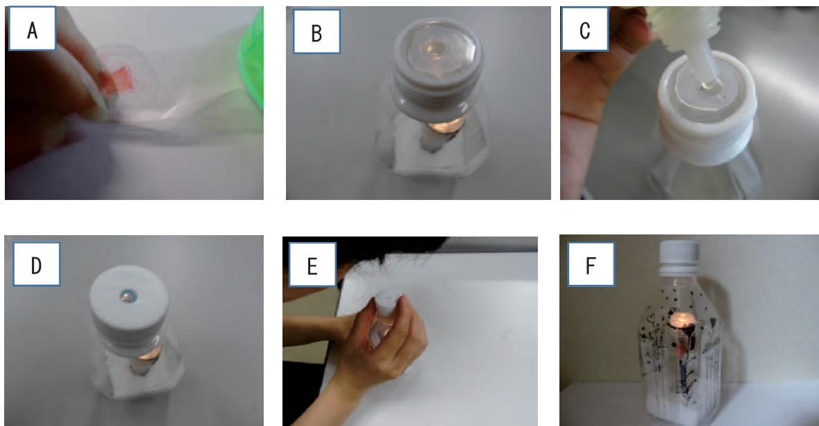
Figure 4. Notes on examination of samples. (A) The dry sample on a piece of scotch tape. (B) The silicone sheet on the top of the plastic cover slip for examining a fluid. (C) The fluid sample at the center. (D) PET bottle cap on top. (E) The sample examination. (F) The bottle decorated for fun
