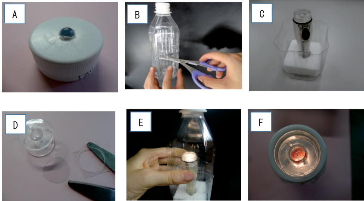
Figure 3. Notes on assembly operation. (A) Acrylic ball placed into the hole. (B) Position for cutting off the base of the bottle. (C) Position of the penlight. (D) The plastic cover slip cut. (E) The top half of the PET bottle fitting into the bottom half. (F) Position of the plastic cover slip.
