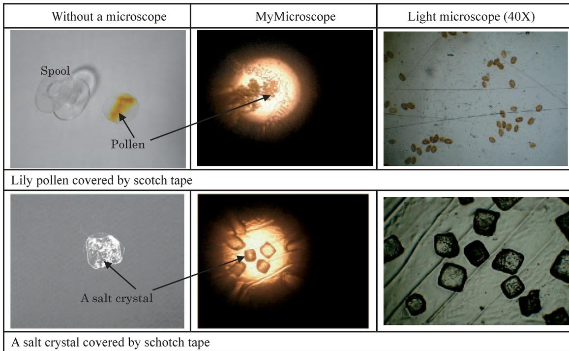
Figure 5. Images of the dry sample through without a microscope, MyMicroscope and light microscope
