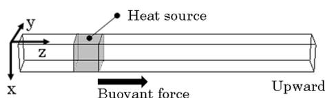
Fig. 1: Computational domain and location of heat source.
