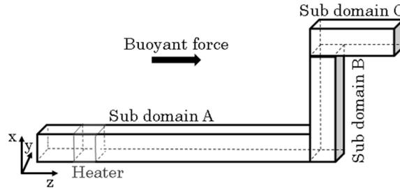
Fig. 3: Orthogonally bended pipes expressed by three sub domains.
