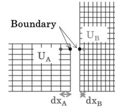
Fig. 5: Connection of sub domains.
