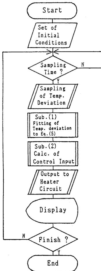
Fig. 2. A simplified flow chart of control programs.
