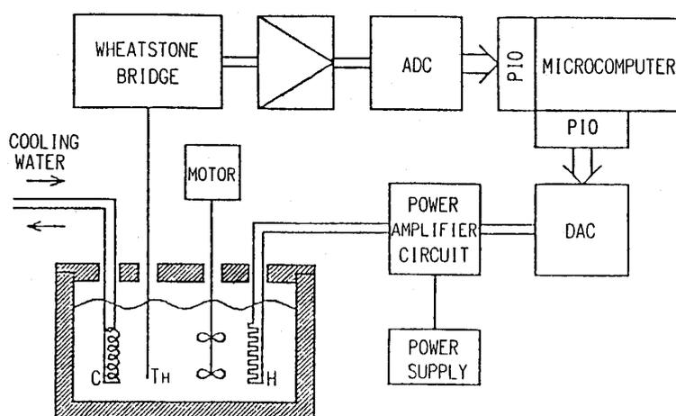
Fig. 1. Schematic diagram of the control system. Th; thermistor, H; heater, C; cooler, ADC; analog-to-digital converter, PIO; programmable parallel input-output, DAC; digital-to-analog converter.
