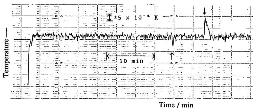
Fig. 5. The typical trace of the controlled temperature of the bath water.
