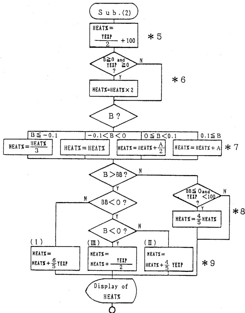
Fig. 4. A flow chart for the calculation of optimal inputs to the heater.
