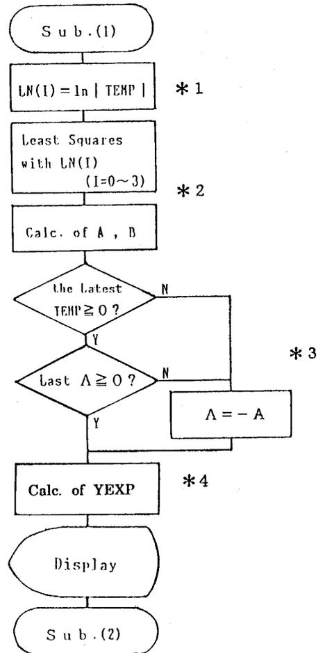
Fig. 3. A flow chart for fitting of the temperature deviations to eqn. (5).
