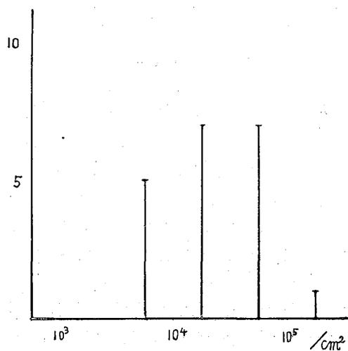
Fig. 6. Distribution of density of pits observed on  $a$ - or  $b$ -face.
