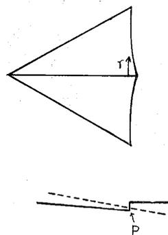
Fig. 9c. Dislocation which makes very small angle with  $\{0001\}$  face.
