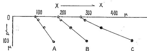
Fig. 3f. Projection of three nearly parallel dislocation lines on the plane, which is defined by  $a$ -axis and  $XX'$ .
