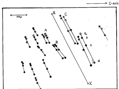
Fig. 3e. Projection of dislocation lines on  $a$ - or  $b$ -plane.
