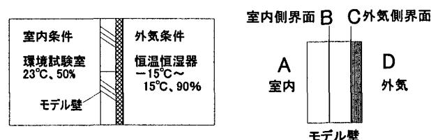
Fig.2 Test installation of the model walls
