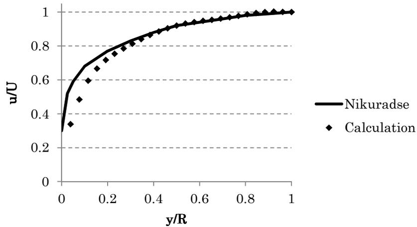
**Fig.4 Velocity distribution in the pipe**
