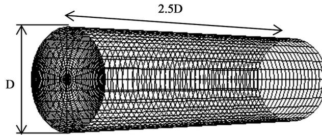
Fig.1 Computational grid of the pipe
