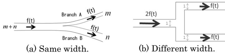
Fig. 2 Schematic figures of flow channel with branches and before them.
