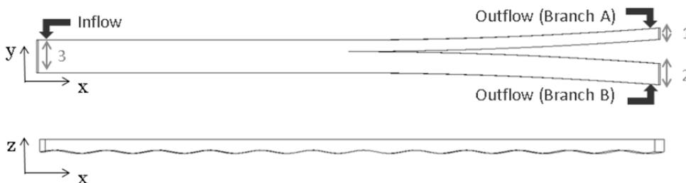
Fig. 10 Computational domain of a channel with branches.
