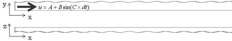
Fig. 7 Computational domain of concave-convex undersurface and one of the side surface.
