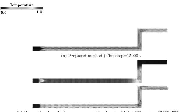
(b) Conventional method, same computational cost with (a) (Timestep=15000, 50000).Fig. 12: Temperature and velocity vector of the pipe.
