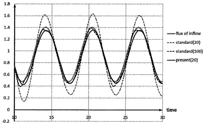
Fig.5(c) Time history of flux of two-dimensional flow in a duct of large curvature
