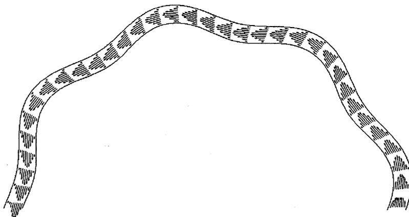
Fig.5 (b) Two-dimensional flow in a duct of large curvature
