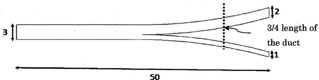
Fig.4(a) The computational domain of a duct with branches.
