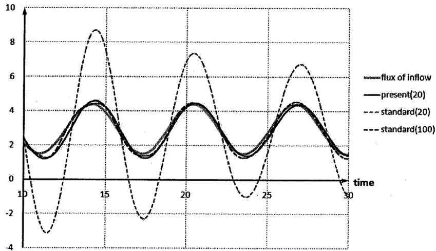
Fig.4(d) The time history of the flux at 3/4 length of the duct with comparison of standard MAC method and the present method. The number noted in bracket represents the iteration number of Poisson equation.
