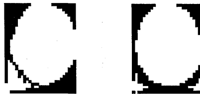
Figure 12: Reconstructions of slant ellipse with maximal prohibited regions; left: from leftmost column; right: from the highest column.
