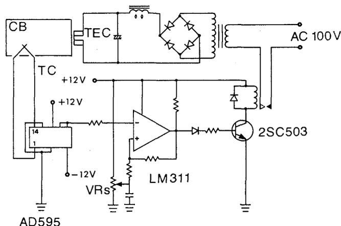
Fig. 1. Electric circuits of temperature control systems. CB; copper board directly cooled by thermoelectric converter (TEC), TC; thermocouple, VRs; a variable resistor which gives a reference voltage for temperature setting.
