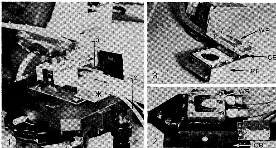
Plate 1. Temperature control devices mounted on a microscope (BHS, Olympus, Tokyo). Two different types of devices are mounted, each of which (indicated by labeled square brackets) is separately shown in Plate 2 or Plate 3. Asterisk indicates the location of a thermocouple amplifier for temperature sensing.
