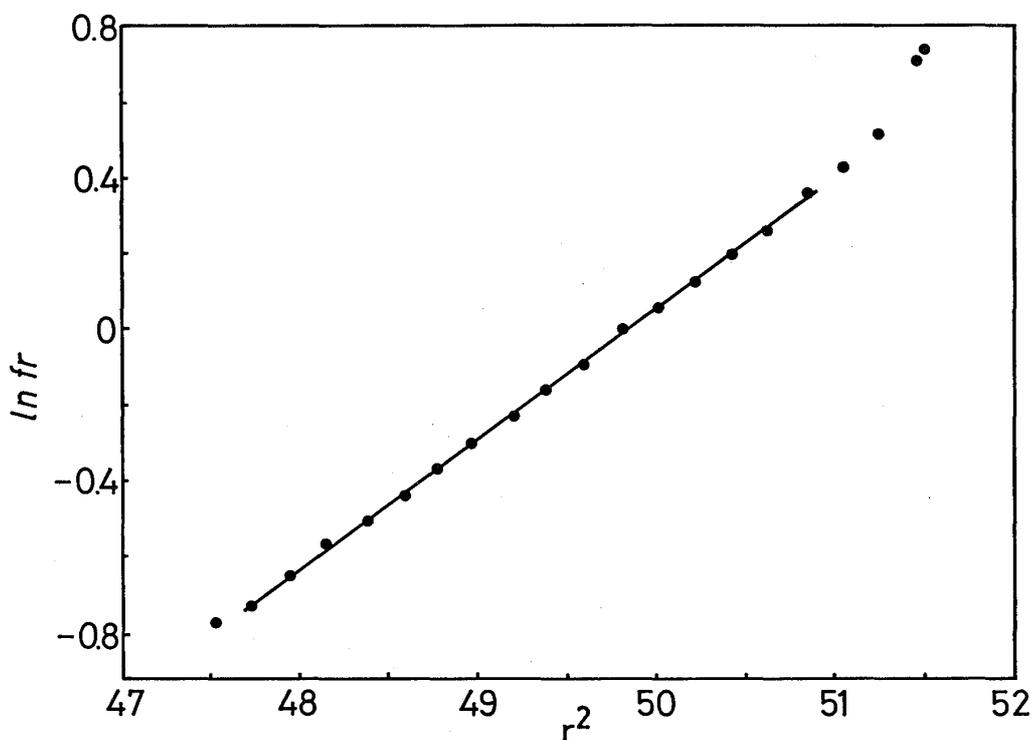
Fig. 2. Sedimentation equilibrium  $\ln fr$  versus  $r^2$  plots. The solution of the lectin in 0.1 M NaCl (3.3 mg/ml) was centrifuged at 8,766 rpm at 19.8°C.
