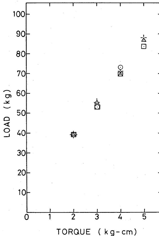
Fig. 2. The relationship between torque and load. Measurements were repeated four times. They were distinguished by square, triangle, circle and cross symbols.
