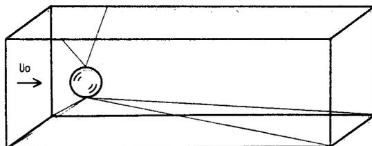
Fig. 3. Sphere fixed to frame by fishing lines.
