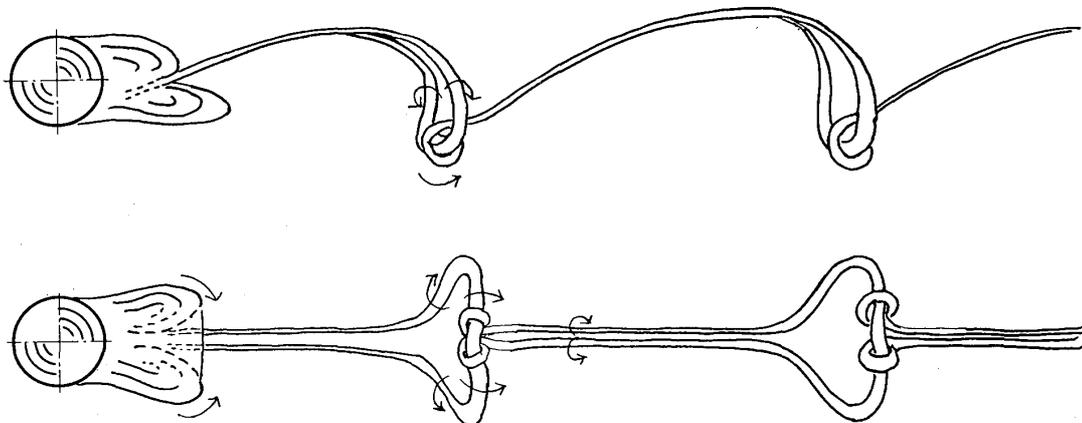
Fig. 5. Schematic representation of the vortex shedding behind the sphere at  $Re=500$ , flow direction is from left to right.
