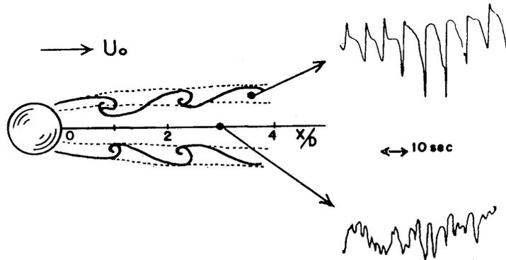
Fig. 7. Flow patterns in the wake of the sphere.
