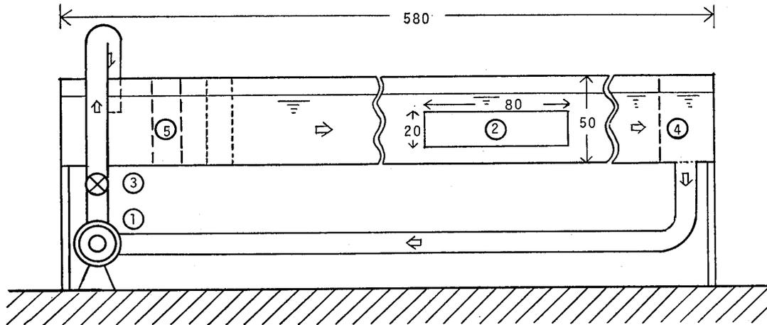
Fig. 1. Circulating water tank, ①: pump, ②: glass plates of test section, ③: controlling valve, ④: slotted plates, ⑤: perforated plates and mesh screens.
