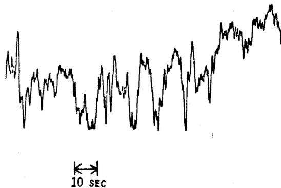
Fig. 9. Flow pattern at  $Re=3680$ ,  $S=1.5$ ,  $S_L=0.13$ .
