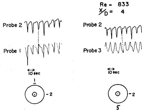
Fig. 8. Flow patterns at different points behind the sphere at the same moment.
