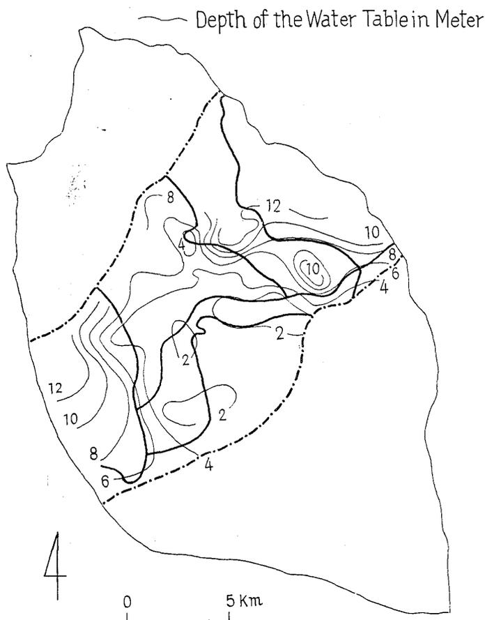
Fig. 6. A map to illustrate the distribution of the depth of the water table by means of the isopleth.
