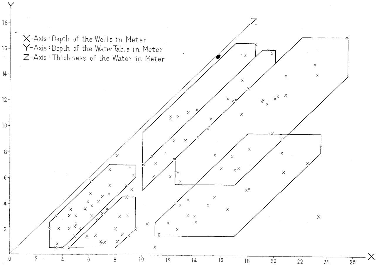
Fig. 1. A coordinate to illustrate the relationships among  $x$ ,  $y$  and  $z$ , i.e. the depth of the wells, the depth of the water table and the thickness of the water in connection with the wells being situated in the central section of the Nasuno-basin, which were surveyed on Oct. 1, 1950. The wells are represented on the coordinate by the symbols  $\times$  and are brought together into six regional groups which are illustrated in Figs. 2 and 3. The  $z$ -axis is explained in the text.
