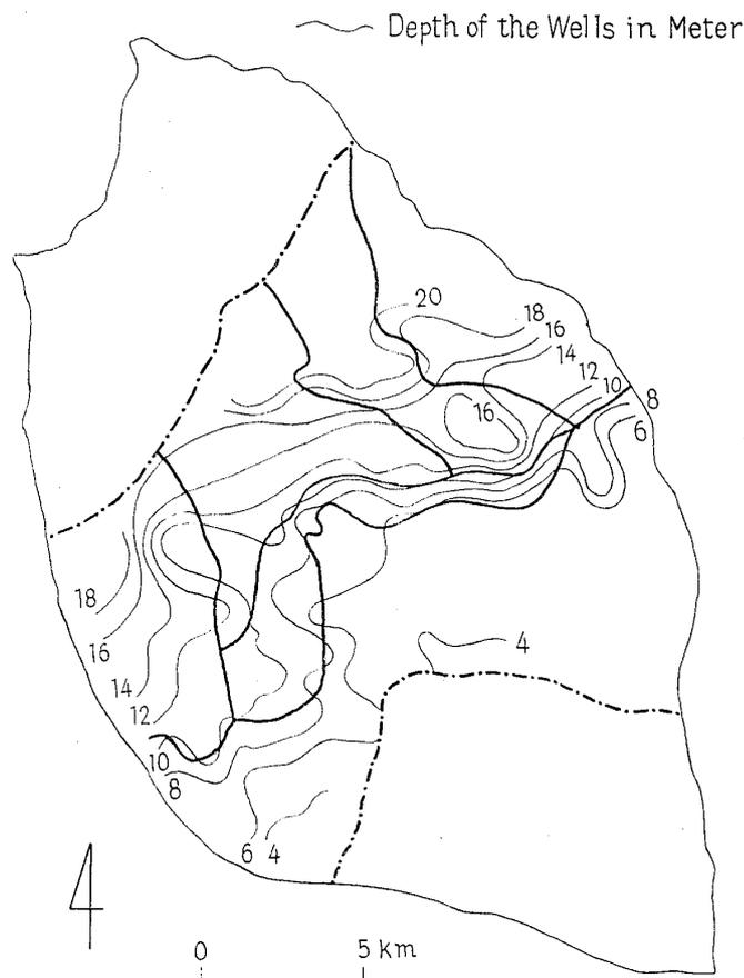
Fig. 4. A map to illustrate the distribution of the depth of the wells, which is represented by means of the isopleth. The boundaries of six subsections are entered in the map. The area of the central section which is taken into consideration is extended, using the survey on Oct. 17, 1961 jointly with the survey on Oct. 1, 1950.
