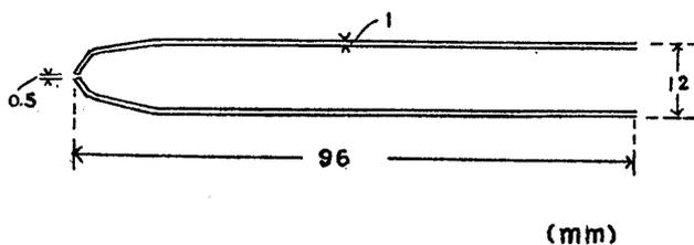
Fig. 1. Leak tube.
