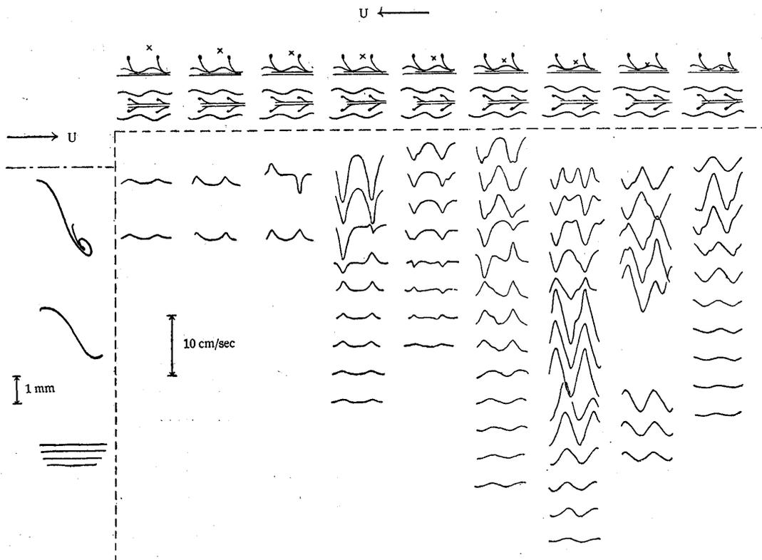
Fig. 11. Wave forms of oscillograms and corresponding positions of hot-wire relative the flow patterns
