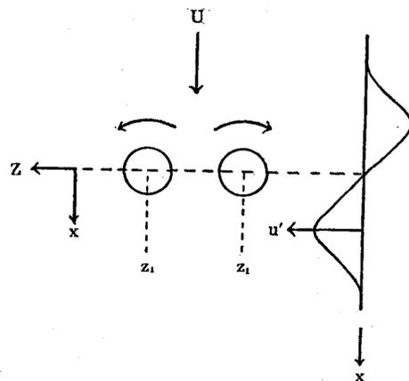
Fig. 8. Distribution of arch-shaped vortices at their legs and resulted velocity profile along  $z = z_1$  or  $z_2$
