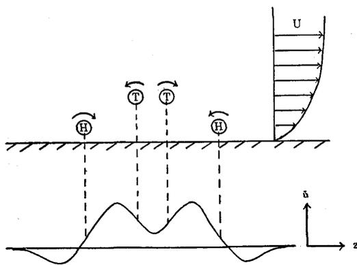
Fig. 7. Distribution of vortices and resulted velocity profiles
