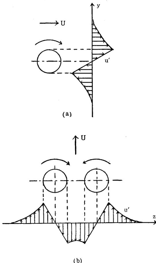
Fig. 12. Profiles of velocity fluctuations caused by (a) a single and (b) a pair of circular vortices
