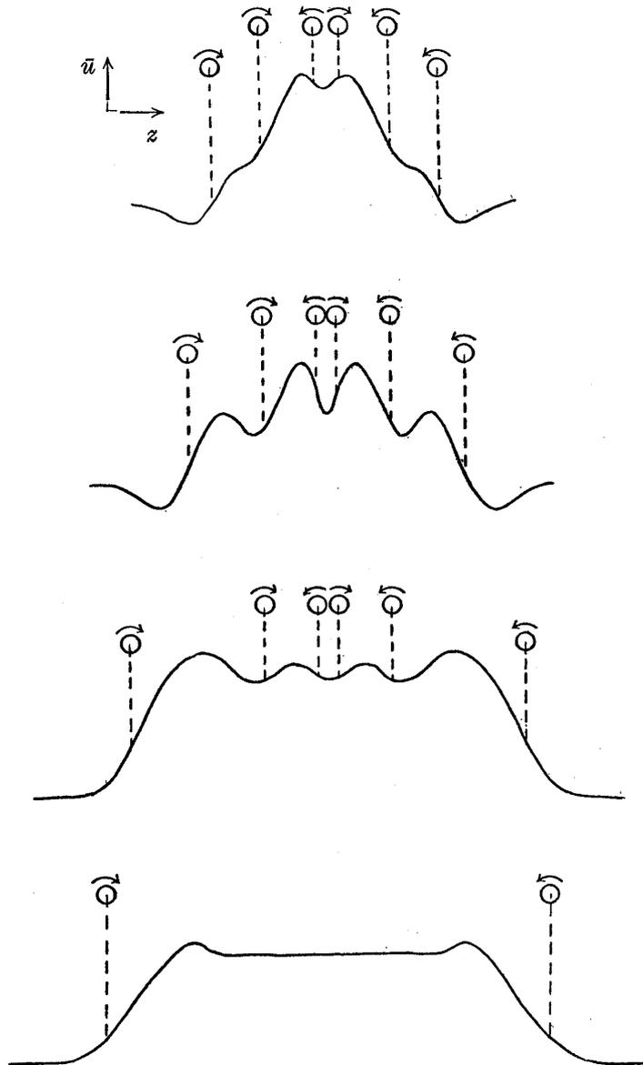
Fig. 9. Distribution of vortices and resulted velocity profiles.
