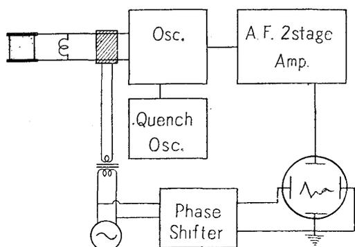
Fig. 1. The block diagram of the superregenerative oscillator.
