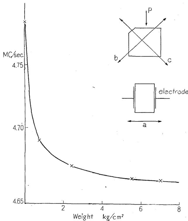
Fig. 8. Pressure versus frequency shift curve observed on the broad line. The section of the crystal is shown with the arrow which indicates the direction of pressure applied.
