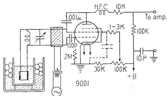
Fig. 2. The circuit of an autodyne oscillator. The cooling device is also shown.
