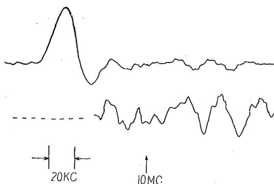
Fig. 4. An example of oscilloscope display. A strong broad line was appeared. Lower pattern shows the fine structure under a high amplification. The broad line was omitted because of saturation of amplifier.
