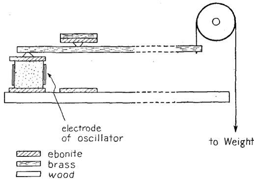
Fig. 7. The schematic diagram of the lever used in pressure effect.
