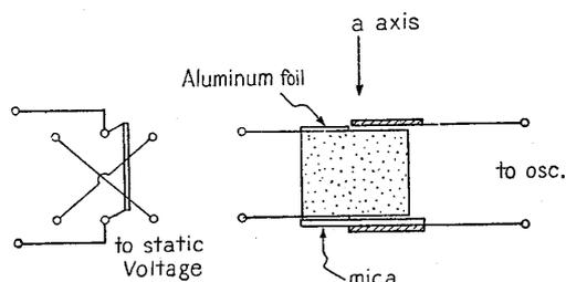
Fig. 9. The arrangement of electrodes in the electrostatic effect.
