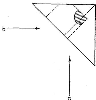
Fig. 3. A single crystal which offered the sample used in various experiments. The sample was cut out along the dotted line. It contains the surface crossed to  $b$  and  $c$  axes with an angle of  $45^\circ$ . The shaded part indicates the possible portion of origin of a strong broad line.
