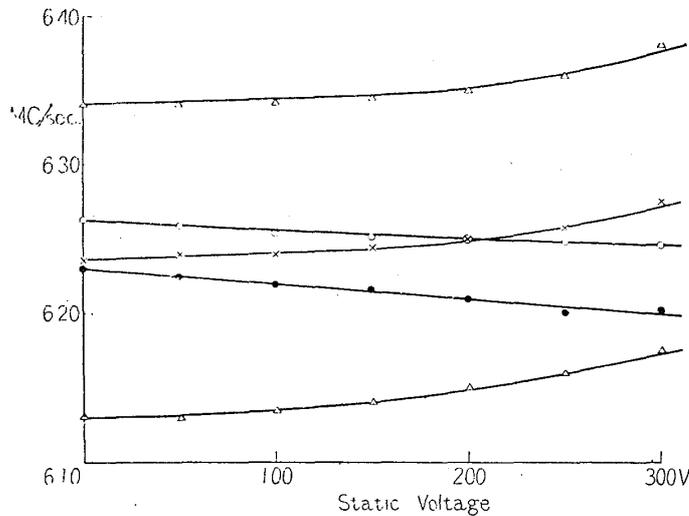
Fig. 10. The frequency shift versus static voltage curves.
