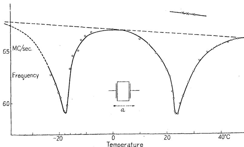
Fig. 6. The temperature versus frequency curves. The high frequency electric field was applied at  $a$  axis.
