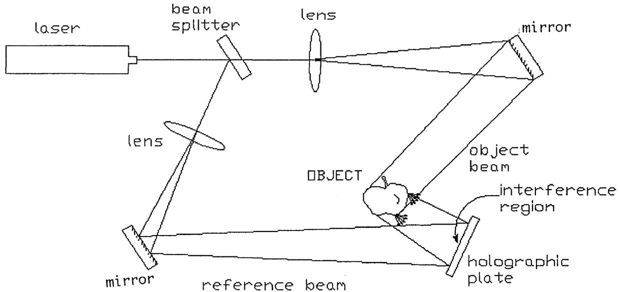
Diagram 1. Optical layout for making a hologram
