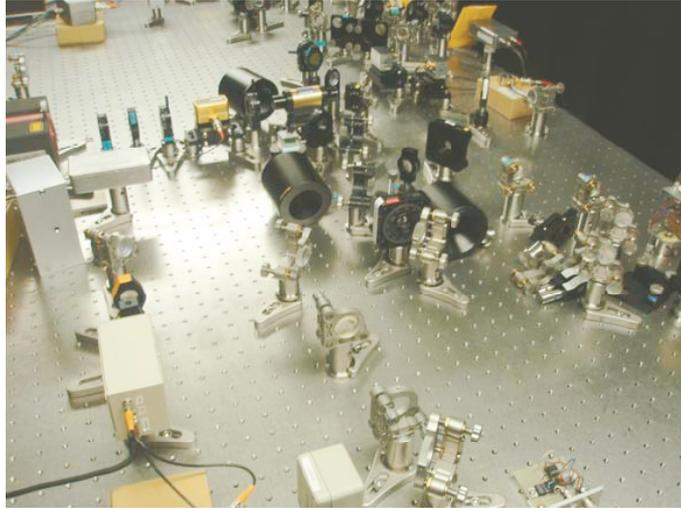
Figure 2: Fabry Perot cavity lock system for verification mirror mounts stability. Cavity could be locked with 20m radius of mirror curvature against the 10cm cavity.
