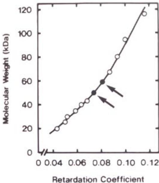
Fig. 4. Standard curve of  $M_r$  against retardation coefficient. Retardation coefficient was the slope of Ferguson plots. Open circles indicate each value of 11 standard proteins listed in Materials and Methods. Closed circles indicated by arrows show two bands of human intact vitronectin. A lower closed circle overlaps an open circle of rabbit IgG heavy chain, one of the standard proteins.
