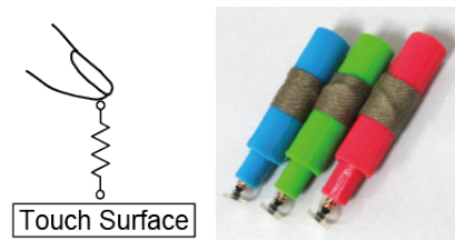
Figure 10. Color Pens with fixed resistors (10 kΩ, 50 kΩ, 100 kΩ).
