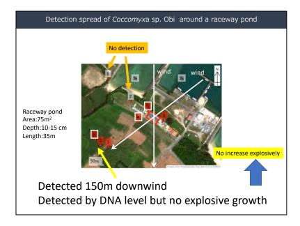
Algae from the raceway pond were detected in the bucket at the point colored red. The raceway pond was situated by the sea and was influenced by north to northeast prevailing winds during winter. The average monthly wind speeds were about 6.0 m/s. You can see the diffusion due to the wind. Also, the algae did not proliferate in large quantities in the bucket and were only detected at the DNA level. No increase explosively.
